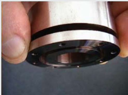
Mirror with mount and 'O' ring groove
