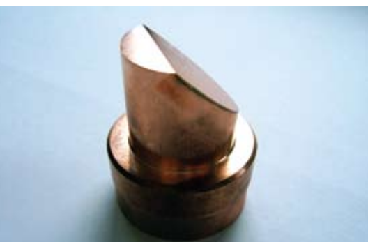
Copper 'lipstick' mirror ready for reworking
