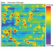
Crystalline mirror surfaces have a grain structure that contributes to scatter and laser damage especially with pulsed lasers. Our amorphous coating eliminates this and dramatically improves pulsed Laser Damage Threshold.
