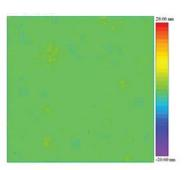
Our polished mirrors have surface roughness around 1/10 of a SPDT mirror. The result is reduced scatter and higher Laser Damage Threshold.
