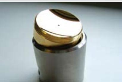
This mirror is a deeply **concave Copper mirror with Gold coating**, used in the infra red for gas sensing. The small central hole is 1mm diameter and the circularity of it was checked with our video microscope. We also made the mounting tube at the same time, guaranteeing the threads mated correctly. Making mirror and mount in one item saves money, reduces assembly time, and simplifies replacement in the field.
