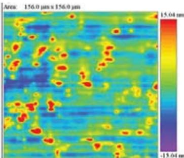
Crystalline mirror surfaces have a grain structure that contributes to scatter and laser damage especially with pulsed lasers. Our amorphous coating eliminates this and dramatically improves pulsed Laser Damage Threshold.
