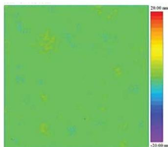
Our polished mirrors have surface roughness around 1/10 of a SPDT mirror. The result is reduced scatter and higher Laser Damage Threshold.
