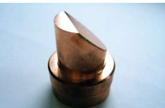
Copper 'lipstick' mirror ready for reworking
