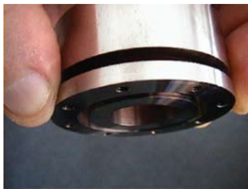
Mirror with mounting holes and O ring groove
