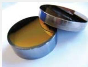
Every metal cutting laser will contain a L/4 phase retarder, sometimes called a 90 degree phase shift or polarising mirror. This mirror circularises the laser beam polarisation to give even cut quality across all axes of motion.
