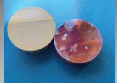
Gold coated Copper (L) and uncoated Copper
