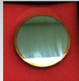
Copper mirror showing pitting marks
