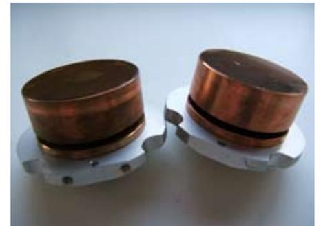
These are internally water cooled zero phase shift beam delivery mirrors.
