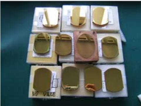
We repolished and recoated these used Copper mirrors from a European car manufacturer saving the customer around 3,000 Euros.
